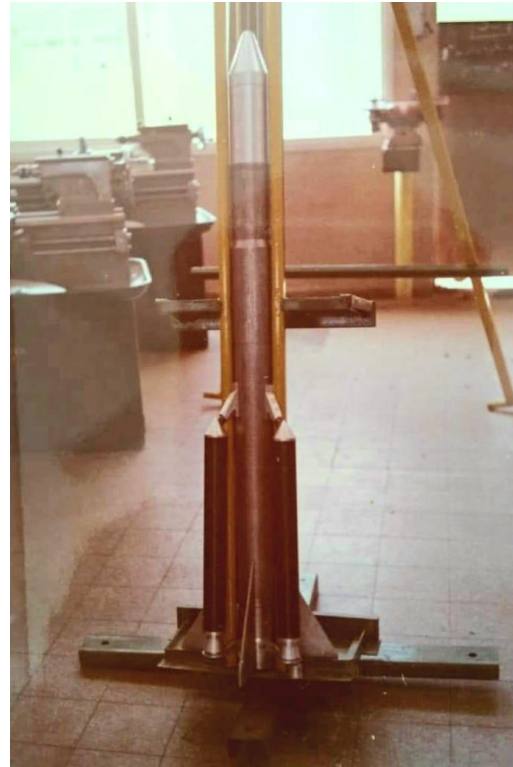
Figure 8: Ort-5 at the workshop- with the boosters attached.
